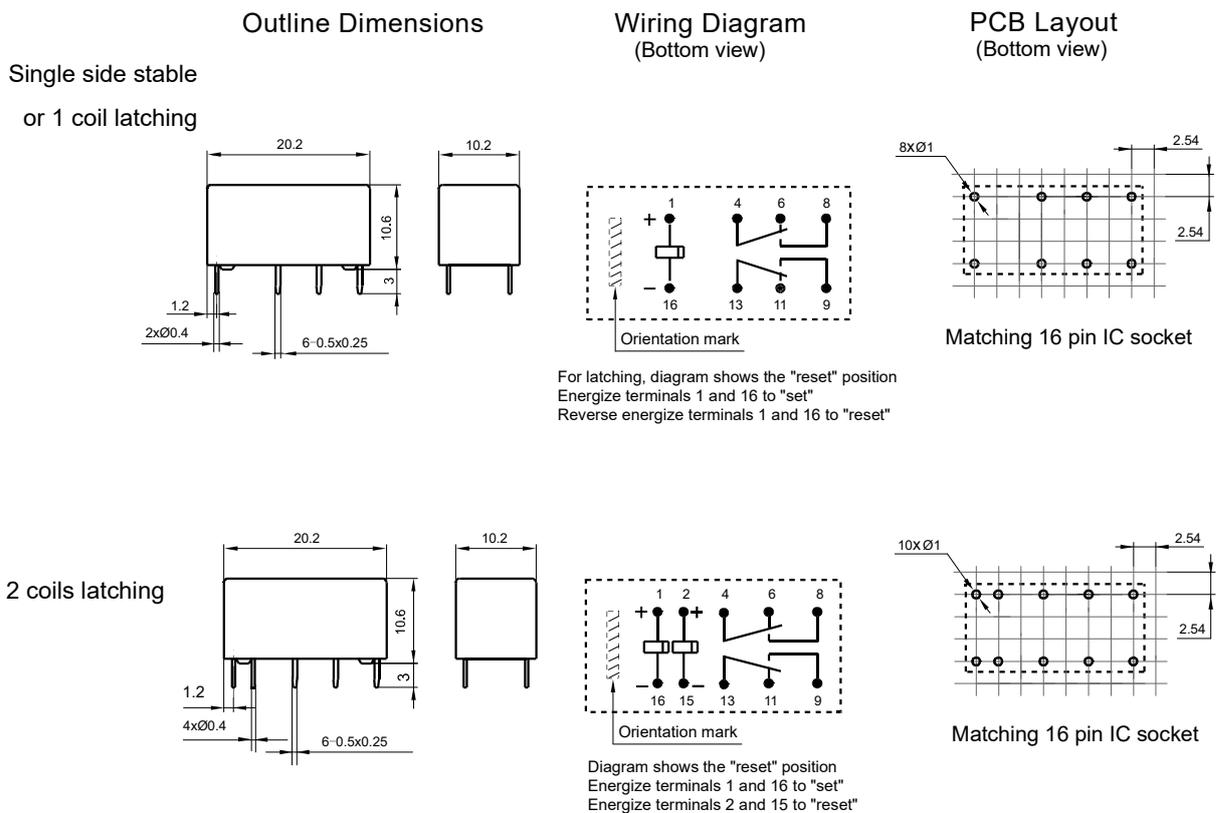
Remark: 1) In case of no tolerance shown in outline dimension: outline dimension  $\leq 1\text{mm}$ , tolerance should be  $\pm 0.2\text{mm}$ ; outline dimension  $> 1\text{mm}$  and  $\leq 5\text{mm}$ , tolerance should be  $\pm 0.3\text{mm}$ ; outline dimension  $> 5\text{mm}$ , tolerance should be  $\pm 0.4\text{mm}$ .
